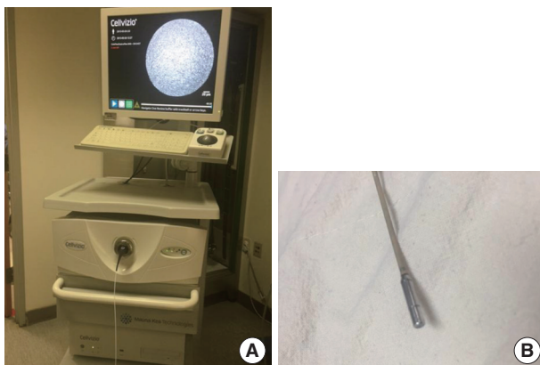
Fig. 4. Cellvizio system for probe based confocal laser endomicroscopy (A) and a probe (B).
